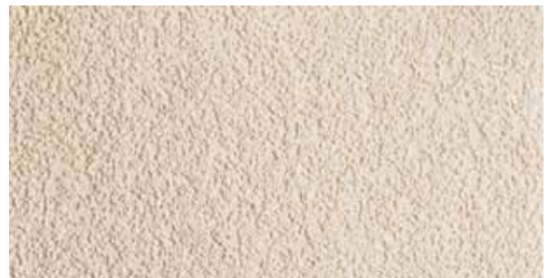
Stone texture produced with Ceresit CT 137 mineral plaster, grain size 2.5 mm, obtained by floating with a plastic float
